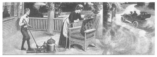
Actual operation of this vacuum was cumbersome at best. It was a heavy, two-person endeavor that required someone to pump the handle to create suction and someone else to direct the wand to the area to be cleaned.
