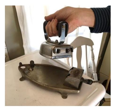
Electricity added a new level of convenience to the chore. Not only were the new electric irons lighter, they had switches to control the temperature of the iron. An early electric iron is shown above. This model had another benefit in that the iron itself was cordless. The base unit held the electric cord and when used, it would heat up the iron to a suitable temperature.
