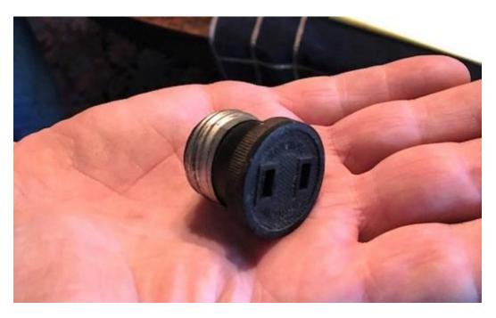
This connection was made possible by removing an incandescent lightbulb from a light fixture and screwing in a lampholder plug to provide an outlet in the room. In the early days it was not uncommon to use a light fixture to power your vacuum cleaner, space heater, flat iron, radio and many other appliances.
