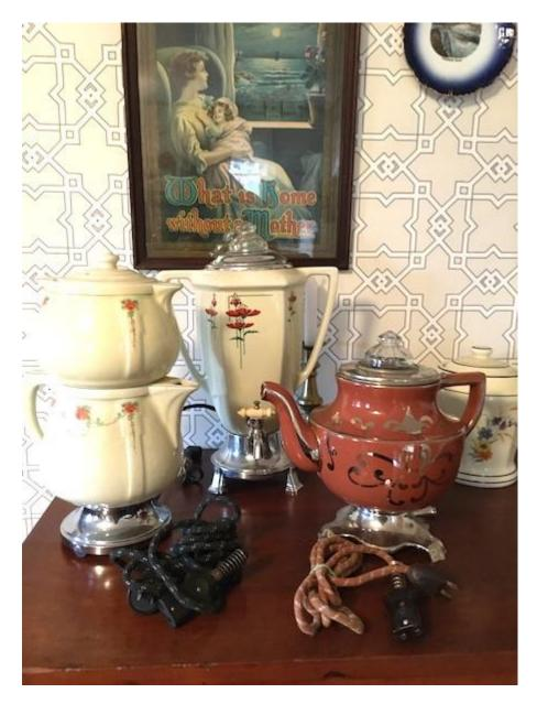
A wide variety of coffee appliances were present in the all-electric home like the Vagg House. The appliance on the left is called a Drip-O-Lator. The coffee maker in the center has a spigot to fill coffee cups, and the ceramic pot on the right is a percolator.
